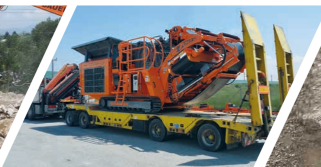
Side conveyor, width: 400 mm / 16" hydraulically foldable Discharge height: ~ 2,2 m / 7'3"
