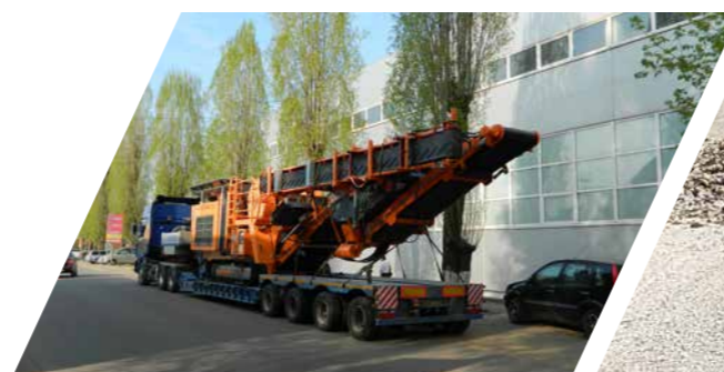
Main conveyor, width: 1000 mm / 40" hydraulically foldable Discharge height: ~ 3,2 m / 10'6"
