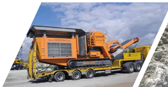
Side conveyor, width: 500 mm / 20" hydraulically foldable Discharge height: ~ 2,2 m / 7'3"
