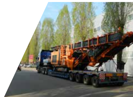
Main conveyor, width: 1000 mm / 40" hydraulically foldable Discharge height: ~ 3,2 m / 10'6"
