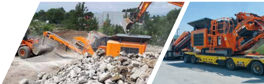
Side conveyor, width: 400 mm / 16" hydraulically foldable Discharge height: ~ 2,2 m / 7'3"
