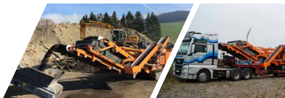
Side conveyor, width: 650 mm / 26" hydraulically foldable Discharge height: ~ 2,4 m / 7'10"
