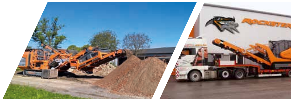
Side conveyor, width: 500 mm / 20" hydraulically foldable Discharge height: ~ 2,3 m / 7'3"
