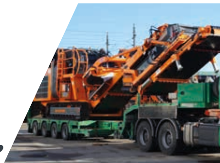
Side conveyor, width: 650 mm / 26" hydraulically foldable Discharge height: ~ 2,4 m / 7'10"
