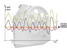
Rockster's hydrostatic drive makes sure that the engine runs in optimum rpm independent from the rotor.
