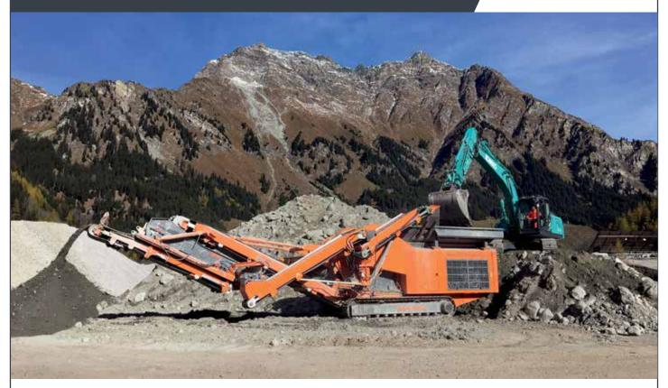
By using the patented Rockster DUPLEX-System with jaw and impact crusher on one basic machine, the Casaccia gravel quarry at the base of the 'Maloja Pass' in Graubünden (Switzerland) can quickly and efficiently meet the diverse requirements of its customers.
