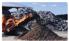
Continuous power to the rotor, independent from the engine, for constant crushing performance.
