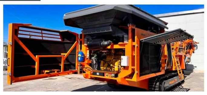
Large covers enable optimal accessibility when it comes to service and maintenance. Furthermore they ensure optimal ventilation of the drive-unit and the cooler.
