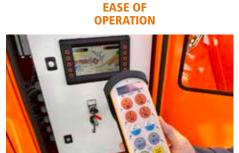
Intuitive easy-to-use central machine control unit with a radio remote control.
