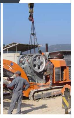
Change the track-mounted impact crusher (R900d) to a jaw crusher (R800) and vice versa - within hours. The machine can be optimized for different requirements depending on the feeding material and because of the
