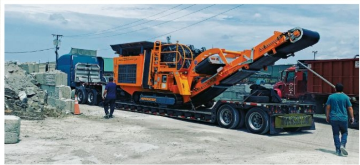
Top: The team at the SC Recycling Center crushes and screens concrete for immediate reuse in Titan Enterprises' road construction projects. Right: The R900 impact crusher weighs 25 tons and is easily transportable, Titan says.
