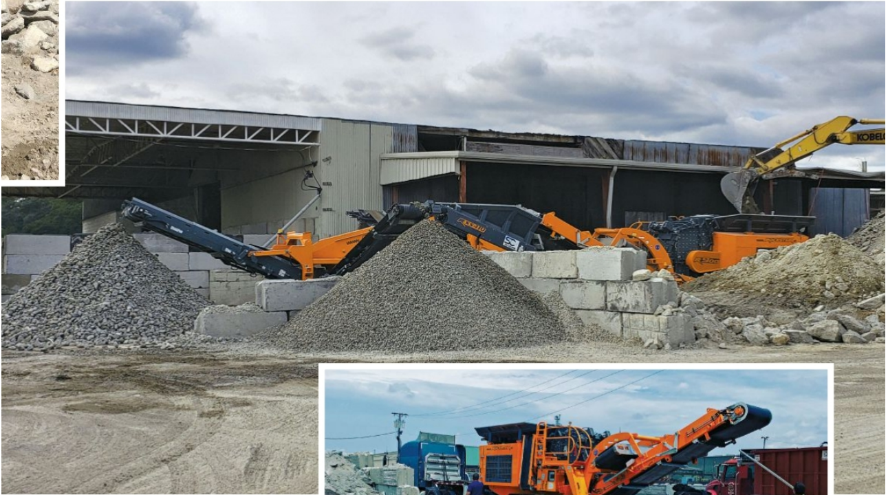
Top: The team at the SC Recycling Center crushes and screens concrete for immediate reuse in Titan Enterprises' road construction projects. Right: The R900 impact crusher weighs 25 tons and is easily transportable, Titan says.
