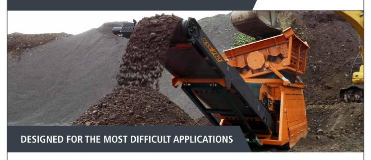
The RSS712 scalping screen is one of the most robust and reliable scalping screens on the market. Built to handle the toughest of applications, the RSS712 comes with a double deck vibrating screen and the longest stockpiling conveyor available.
