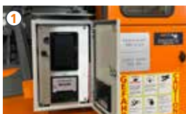
Belt weigh scale incl. printer
